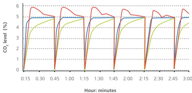
Precisely-tuned sensor and software result in fast recovery of CO<sub>2</sub> without overshoot. This ensures uniform CO<sub>2</sub> levels even with frequent incubator door opening.
