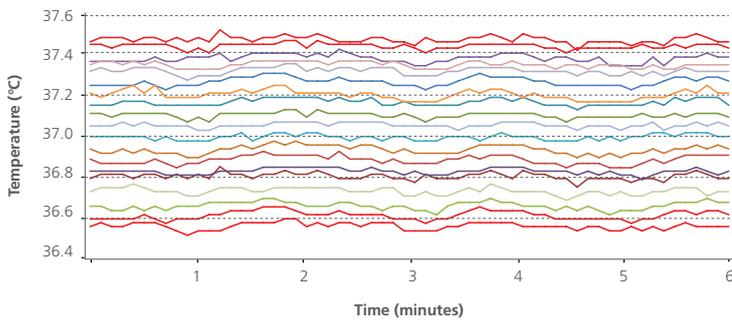
Different lines represent different sensor positions inside the chamber. Esco CelCulture® has uniformity variance of less than  $\pm 0.5^\circ\text{C}$  which means all the samples are evenly heated.\*
