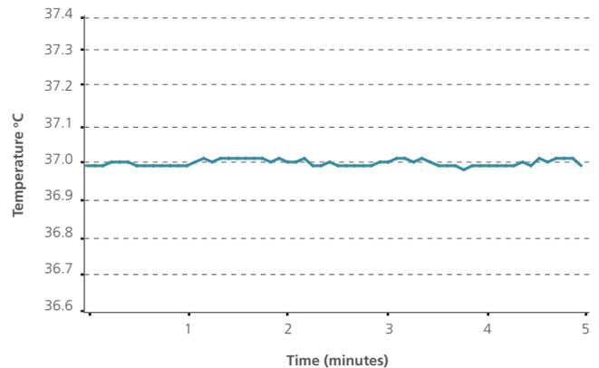
Minimal fluctuation ( $\pm 0.2^\circ\text{C}$ ) ensures temperature stability.\*
